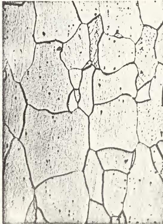
FIG. 27 AT 540°C, UNDER .005%/HR. STRAIN RATE, FOR 30 HOURS (ROCKWELL 30T 33.6)
